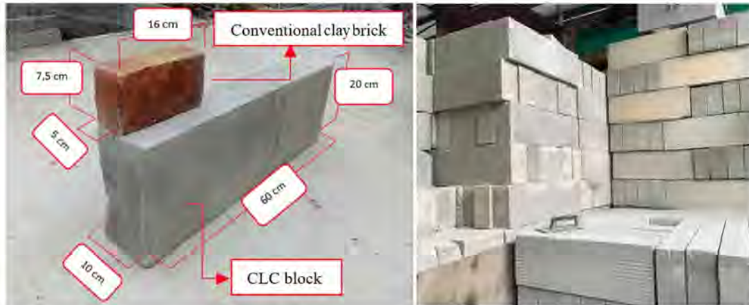
Figure 1. Cellular Lightweight Concrete blocks (a) size comparison with conventional clay brick (b) set of hardened CLC
