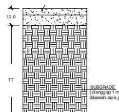
$$\begin{aligned} H\text{-asp} &: 10 \text{ cm} \\ Mr &: 79.516,571 \text{ Kpa} \\ Ep &: 8.557.669,434 \text{ Kpa} \\ \mu &: 0,35 \text{ dan } 0,45 \end{aligned}$$
