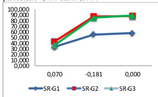
**Gambar** Error! No text of specified style in document..**11** Perbandingan Sudut Geser Antara Gradiasi Pasir Sub-rounded.
