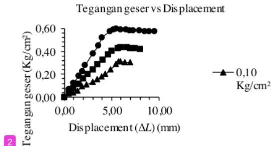
**Gambar** Error! No text of specified style in document..2 Grafik Tegangan Geser VS Displacement (SA-G17)
