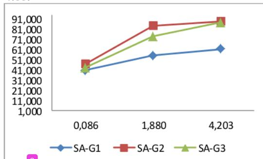
2 Gambar Error! No text of specified style in document..10 Perbandingan Sudut Geser Antara Gradiasi Pasir Sub-angular.
