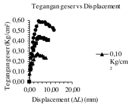
**Gambar** Error! No text of specified style in document..4 Grafik Tegangan Geser VS Displacement (SA-G1 14).
