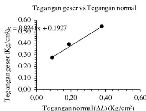
6 Gambar Error! No text of specified style in document..9 Grafik Tegangan Geser VS Tegangan Normal (SR-G1 14).
