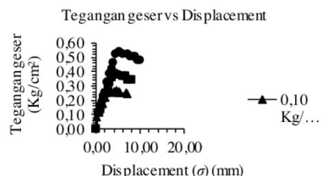
2 Gambar Error! No text of specified style in document..8 Grafik Tegangan Geser VS Displacement (SR-G1 14).
